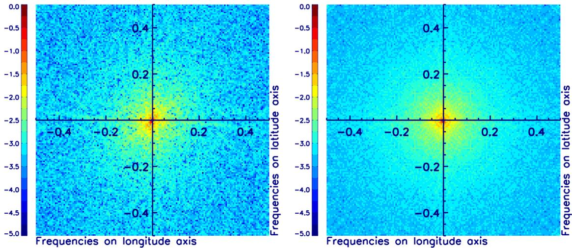
Fig.2 : left : base 10 logarithm of the Bi-Fourier spectrum resulting from the FFT computation on the indicator field. right : Bi-Fourier spectrum smoothed after isotropy assumption.
